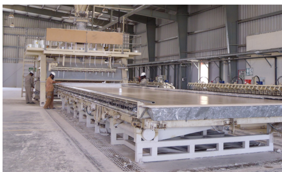
Rapidwall panel manufacture
