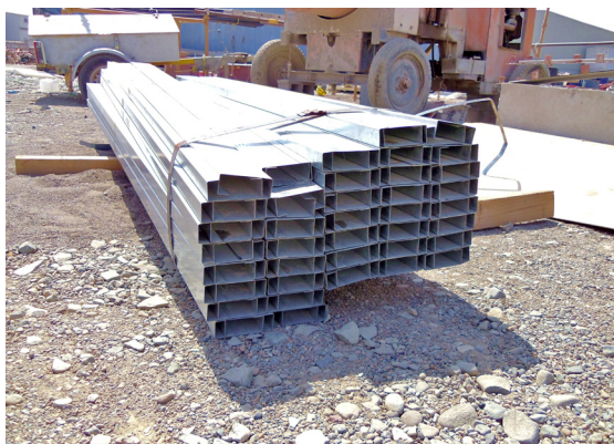
Metal studs: 92mm x 135mm x 1.15 bmt
