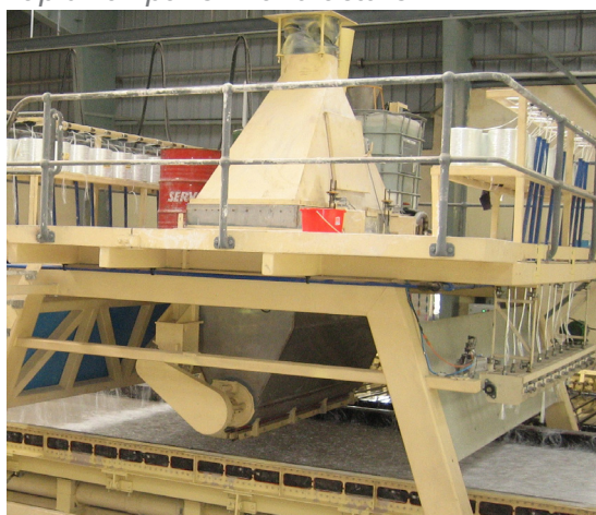
Laying fibreglass during manufacture
