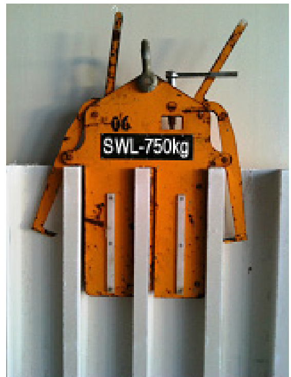
Lifting jaw showing clamping method
