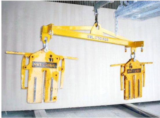
Lifting jaws set up on spreader bar
